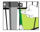
3. Clip together with the fence strip mount onto the end of each panel.
